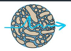
The aquifers of most interest to us in the Mississippi embayment are comprised of sand, gravel, silt and clay, but it is the sands and gravels that really provide us the water we need. Water moves through the **porous media**, or the interconnection of voids between the grains. Sometimes the water finds it easy to move, other times not – that's **hydraulic conductivity!**
